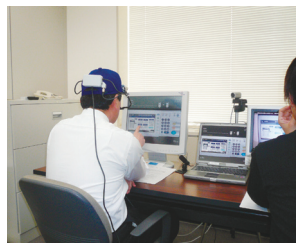
Experiments conducted to check usability of the operation screen, using the eye movement measuring apparatus or eye camera
