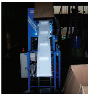
Fig 1. A shredder fed with an input conveyor is used to break up the bottles and cartridges. Also, some toner can be reclaimed at this step.
