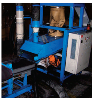
Fig 2. A magnetic separator is used to remove any iron-based parts with a safety additional magnet at conveyor output for safety
