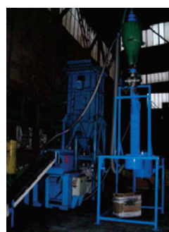
Fig 4. By using a "Zig-zag" tower, any remaining unwanted contaminants such as labels, dust and toner are removed.
