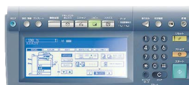
Application of easy-to-see large display panel and large buttons
