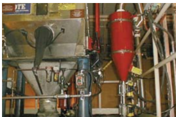
Toner Tote Tilt and Newly Installed Vacuum Receiver
