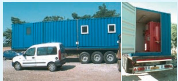
Container truck equipped with a grinder
