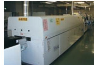
Lead-free soldering facility (reflow soldering)
