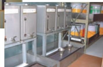
"No Leakage Allowed" management using the leakage preventing facility
