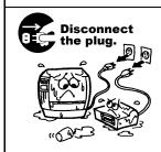
If foreign objects (metal fragments, water, liquids) enter the machine, turn off the power switch and disconnect the power cord plug from the outlet, and then contact your authorised TOSHIBA TEC CORPORATION representative for assistance. Continued use of the machine in that condition may cause fire or electric shock.
