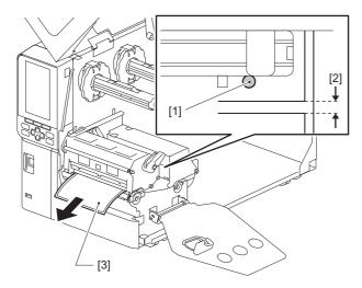
**5** Manually position the media sensor [1] to ensure the transmissive sensor's indicator (•) [2] precisely aligns with the required gap.
