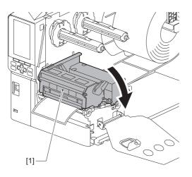
**12** Set the ribbon shaft fixing plate [1] and secure the print head block by rotating the head lever [2] to the "LABEL" or "TAG" position, depending on the media type.
