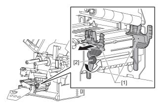
**9** Pass the leading edge of the media [1] between the left and right media guides [2], and feed it to the media outlet through the lower side of the print head block.
