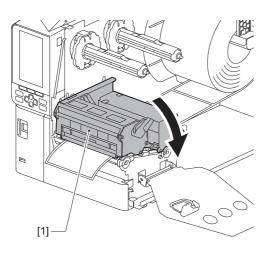
6 Install the ribbon shaft fixing plate [1] and then turn the head lever [2] to the "LABEL" or "TAG" position to secure the print head block, depending on the media you are using.
