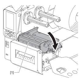
4 Set the ribbon shaft fixing plate [1] and secure the print head block by rotating the head lever [2] to the "LABEL" or "TAG" position, depending on the media type.
