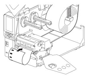
**5** Move the media sensor [1] by hand and align the reflective sensor [2] with the center line of the black mark [3].
