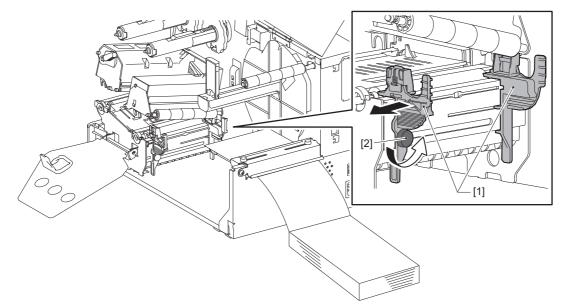
8 Pass the leading edge of the media [1] between the left and right media guides [2], and feed it to the media outlet through the lower side of the print head block.
