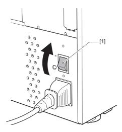
**2** Press the POWER button [1] on the front of the printer.
