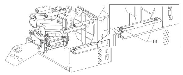
**5** Place fanfold paper [1] behind the rear of the printer and insert the end of it into the media slot under the external media guide [2].
