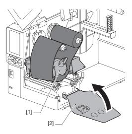
8 Turn the ribbon shaft [1] on the take-up side clockwise to fully wind up the leader tape section (silver) [2] on the ribbon.
