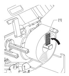
8 Loosen the thumbscrew [2] on the media guides [1] and spread them slightly wider than the width of the media.
