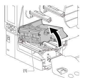
**5** Wipe dirt off the platen unit [1] a soft cloth containing a small amount of anhydrous ethanol. Conduct cleaning for each roll of media.
