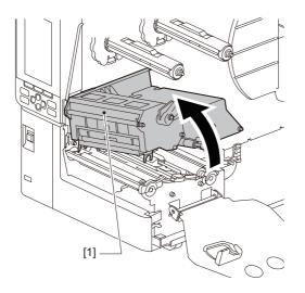
**5** Clean the pinch roller [1] and feed roller [2] with a soft cloth containing a small amount of anhydrous ethanol.
