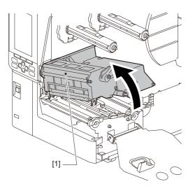
5 Clean the media detection sensor [1] and the ribbon end sensor [2] with a soft cloth containing a small amount of anhydrous ethanol or a cotton swab. Wipe paper powder and dust with a dry, soft cloth.
