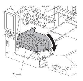
**11** Set the ribbon shaft fixing plate [1] and secure the print head block by rotating the head lever [2] to the "LABEL" or "TAG" position, depending on the media type.
