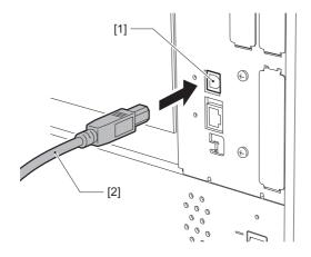
**4 Connect the connector on the other end of the USB cable to the USB interface on the computer.** Refer to the owner's manual for the computer being used regarding how to connect to the computer.
