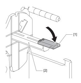
**5** Set the media on the supply shaft [1], and pass the media behind the media guide shaft [2].
