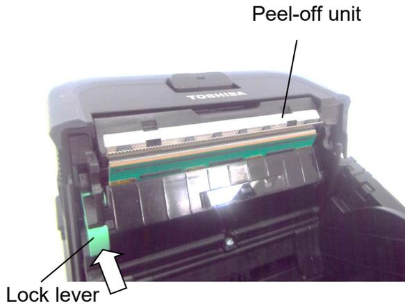
2. The peel-off unit is lifted. Refer to "Loading the Media" on the previous page and set a label roll.
