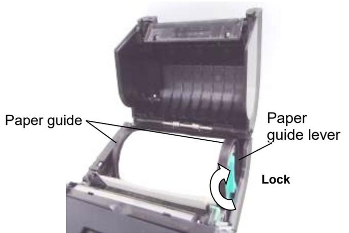
6. Pull the top edge of the media toward the operation panel, and close the top cover removing slack of the media.
