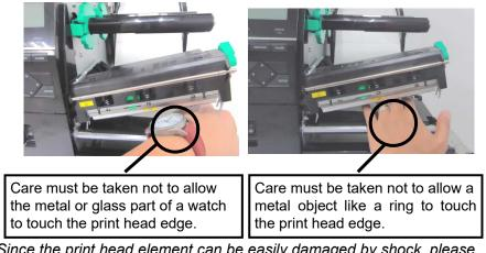
Since the print head element can be easily damaged by shock, please treat it carefully and do not hit it with hard objects.
