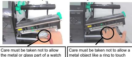
the metal or glass part of a watch<br/>to touch the print head.metal object like a ring to touch<br/>the print head.Since the print head element can be easily damaged by shock, please
