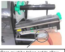
Care must be taken not to allow the metal or glass part of a watch to touch the print head edge.
