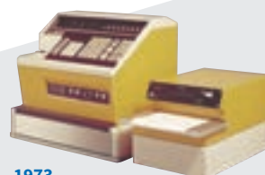
1973 Microcomputer chip-incorporated BRC-32CF-GS electronic accounting machine
