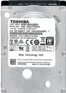
An HDD (hard disk device) is equipped in TOSHIBA MFPs with the e-BRIDGE controller installed. Scanned original document data in copying are stored temporarily in the HDD. When copying is completed, although the management information (FAT: File Allocation Table) is erased, the temporarily stored data still remain in the HDD. In addition, a confidential document can be stored and controlled with a password in an e-Filing box of the HDD.
