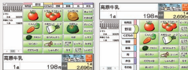
Visibility and operating efficiency improved by flexible screen configuration allowing for checker's line of sight and personal layout preferences
