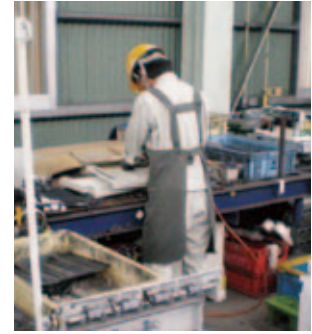
Manual disassembly of a MFP
