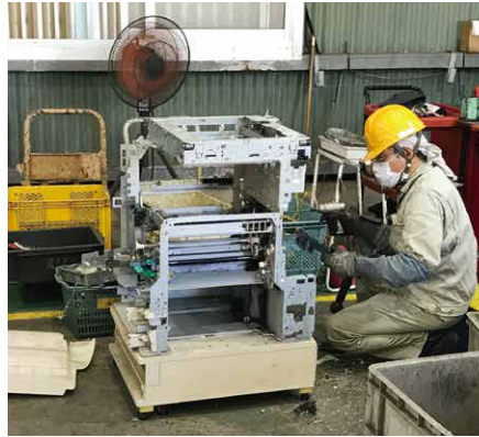
Dismantling a MFP
