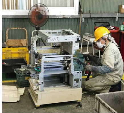
Dismantling a MFP
